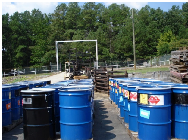
Maintain proper aisle space.
