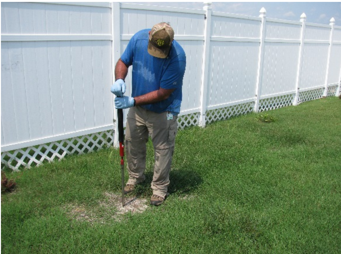
ADEM Personnel Performing Soil Sampling and GPS Locating At Emerson Buried Drum Site, Montgomery, AL
