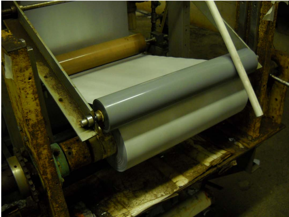
Aluminum foil rolls in etching machine
