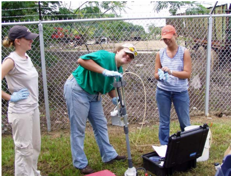
Groundwater Sampling Utilizing Manual Bladder Pump Montgomery Brownfield, Montgomery, AL
