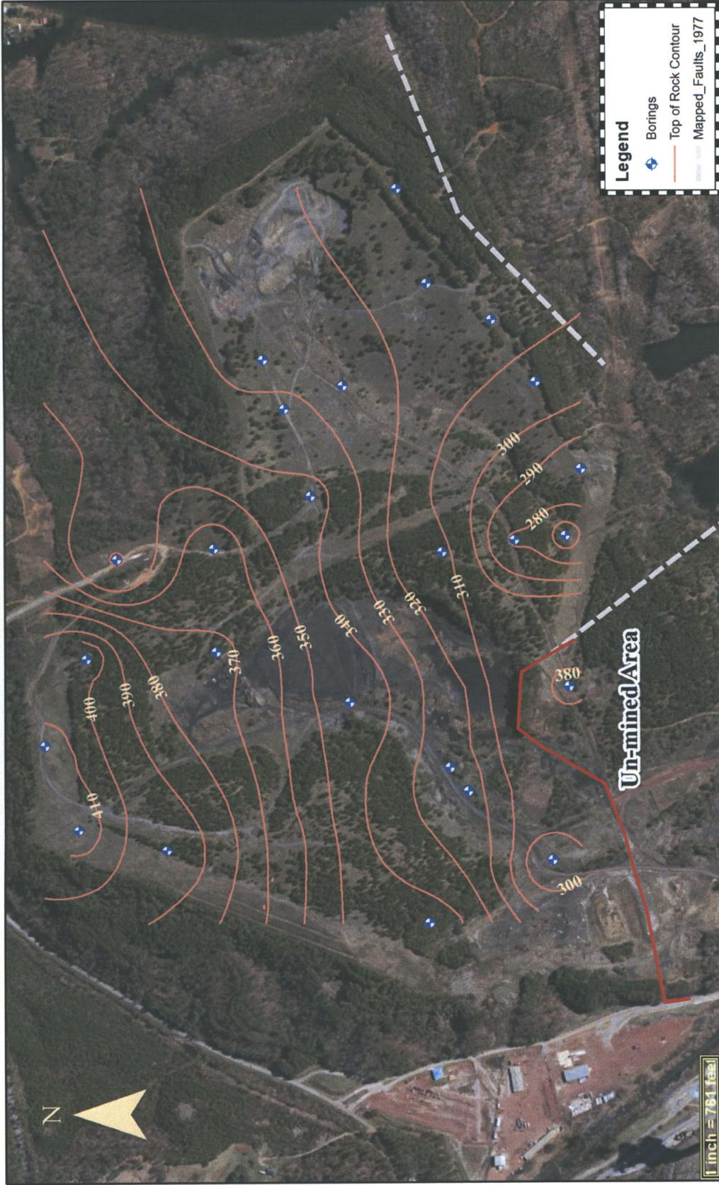
Figure 5-4. Top of Rock Structural Contours
