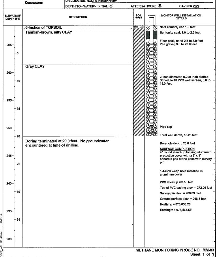
METHANE MONITORING PROBE NO. MM-83 Sheet 1 of 1
