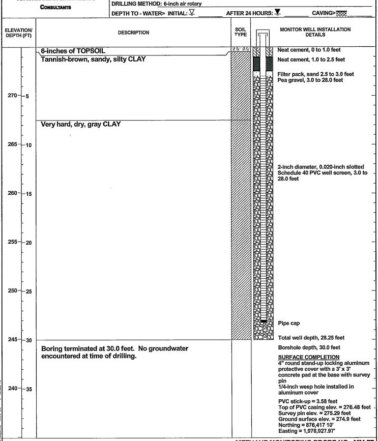
METHANE MONITORING PROBE NO. MM-77
