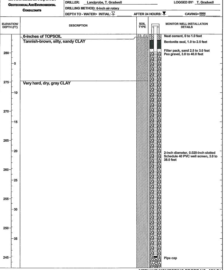
METHANE MONITORING PROBE NO. MM-74
