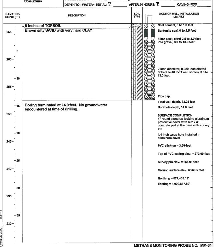
METHANE MONITORING PROBE NO. MM-64 Sheet 1 of 1
