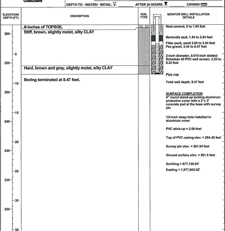
METHANE MONITORING PROBE NO. MM-91 Sheet 1 of 1
